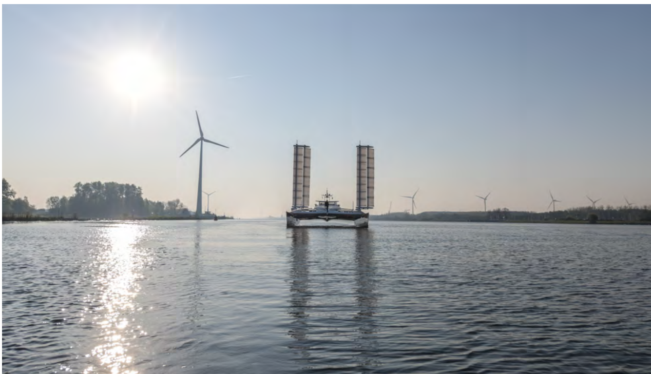
Energy Observer 2019: 27m 2 more solar panels, increased thermal storage and two Oceanwings wings to provide greater speed and produce hydrogen by electrolysis of sea water. A new energy model.
